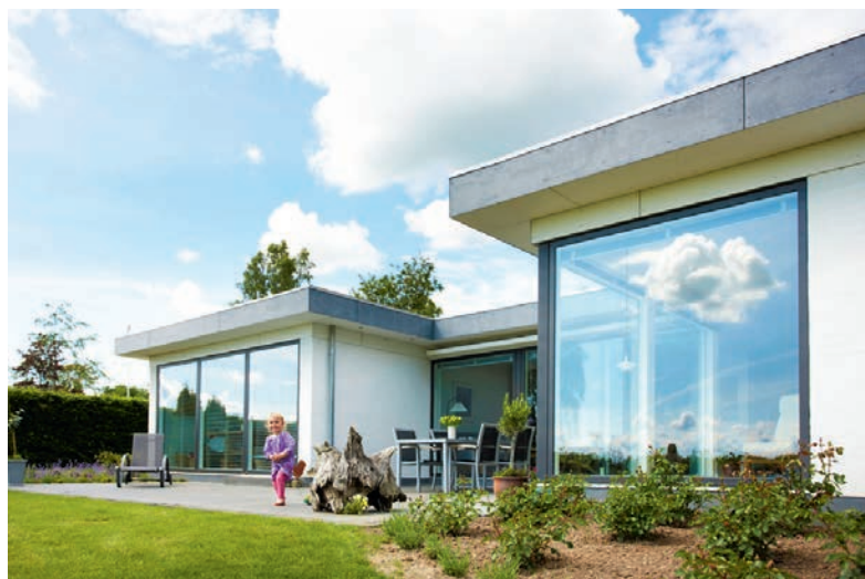
Above: Velfac's 200 series of composite aluminium-timber windows and patio doors feature uniform sightlines, and are available in both double and triple-glazed formats
