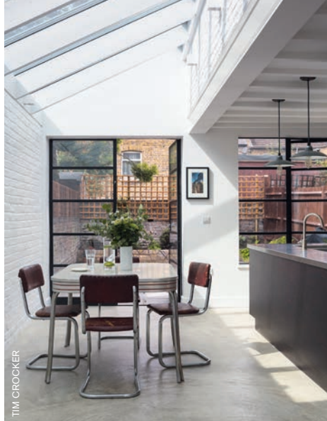
Left: This side-return extension by Mustard Architects features triple-glazed rooflights with a solar control coating to maximise natural light while maintaining a comfortable year-round temperature
